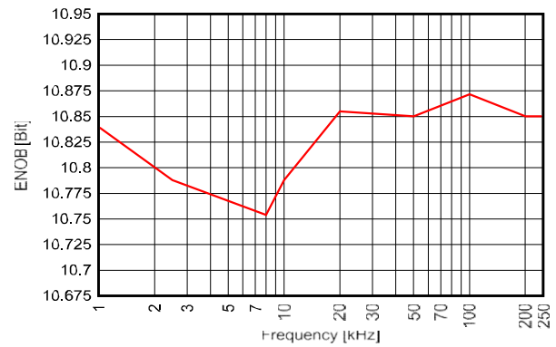
Figure 7-28. ENOB vs. Sampling Frequency ( V_{in} = 3V Sine Wave, Internal Reference, F_{in}=F_s/10 )
