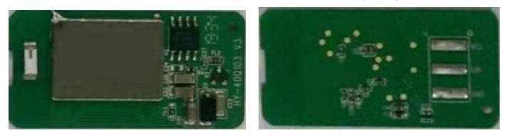
5.HY-40Q103 V2 LIN bus Bluetooth Vechile Spec. block size picture & pin picture PCBA size: 40\*20\*4.0mm
