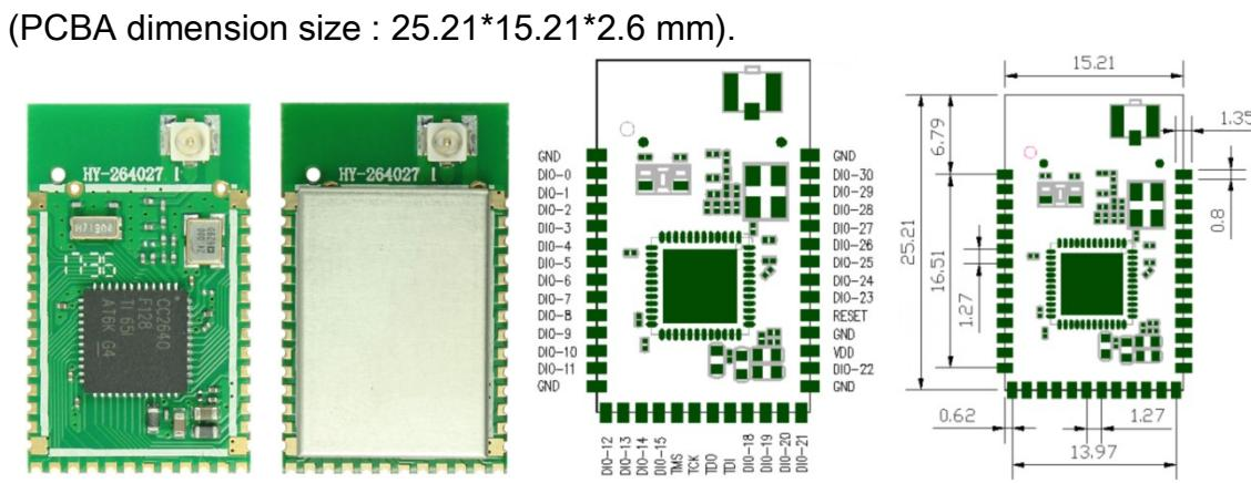
3-3: HY-264027W / WMD400027SR6W0( Metal WireAntenna)(1/4λ half wave dipole)\_
